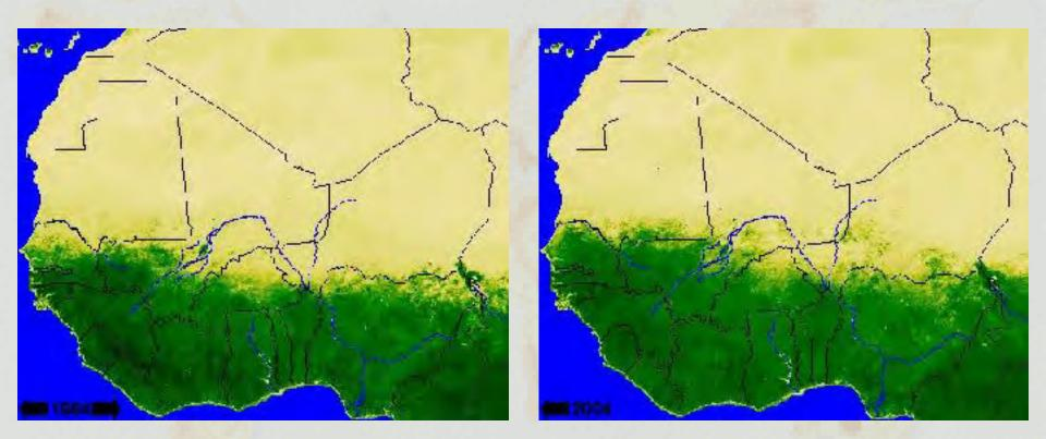
In time series analysis of NDVI images it is common to use either monthly or annual maximum value compositions. This is a way to Make sure that cloud contamination is kept at a minimum.
