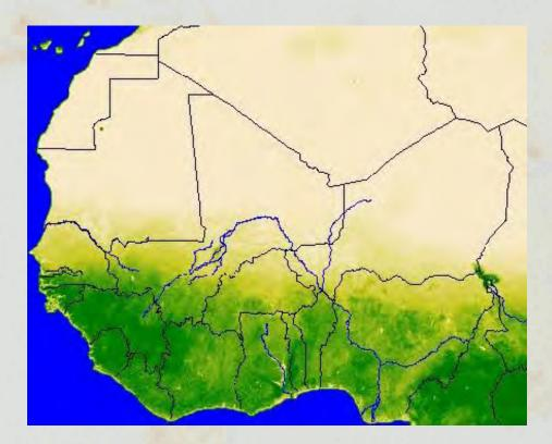
The GIMMS NDVI data is at 8 km spatial resolution. Preprocessing of the includes corrections for sensor degradation, for satellite orbital drift and for atmospheric volcanic aerosols from eruptions in 1982 and 1991. The data is then agglomerated to 10-day composite using a maximum value compositing procedure to minimize the effects of cloud contamination.
