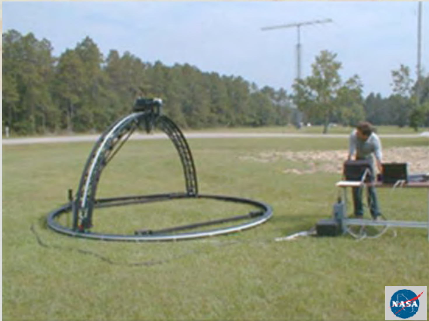
The Sandmeier Field Goniometer; A measurement Tool for Bi-directional reflectance.
