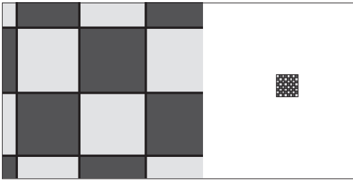
Figure 2. Two raster data sets with different grain size. The ease with which you will be able to understand chess will obviously be dependent on the resolution or grain size used to capture the chessboard
