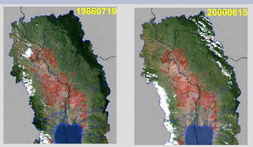
Landsat images over Rusizi River showing the potential hotspot areas identified from the compound index based on time-series analysis of NDVI and EVI. Thomas Gumbricht, ICRAF, 20100701
