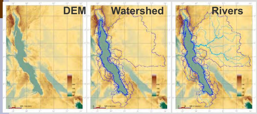
The Digital Elevation Model was used to create maps of watersheds and streams.
