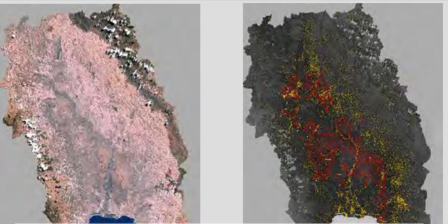
The image to the left shows the soil surface with the vegetation "removed", the spectral properties of the soil in the Rusizi Delta was then used to try to find soil with a similar spectral signal in the Rusizi watershed – the image to the right.
