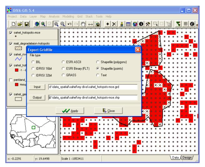
From the illustration above you can see that each cell from the grid is exported as a feature in the new shapefile (points in the example). The generated shapefile will hence have as many features as there are cells in the grid file, and will be very slow to work with (if you try to symbolize this vector file it will take a very long time for DIVA-GIS to process it).
