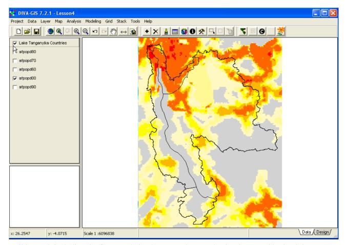
Build a stack including the five population layers. Make sure the data is entered in the right sequence with the oldest population data coming first and the most recent last in the stack, as shown below.
